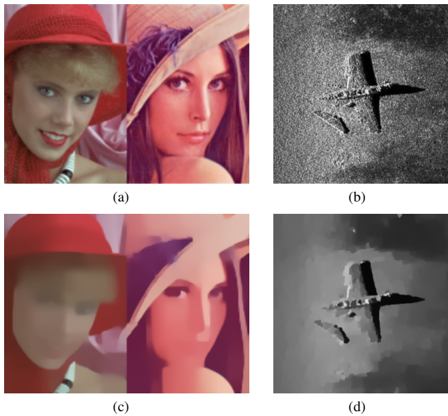
Fig. 4. A sonar image and a NSI without detailed information, which shows the importance of macroscopic structure in a sonar image. (a) Original NSI “Woman”; (b) Original sonar image “Aircraft Wreckage”; (c) “Woman” without microscopic structures; and (d) “Aircraft Wreckage” without microscopic structures.
