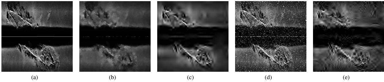
Fig. 2. Examples of sonar images in the SIQD database, which demonstrate the typical distortion types contained in the SIQD database. (a) Reference image; (b) Distorted sonar image with ‘CC’, MOS=35.15; (c) Distorted sonar image with ‘CS’, MOS=32.34; (d) Distorted sonar image with ‘TC’, MOS=34.21; and (e) Distorted sonar image with ‘TS’, MOS=35.01.
